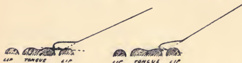
FIG. 2. In the above diagram the hooks are shown in an upright position. In practice they will generally be inclined over on their sides, which would make the necessity for a searching point to be still greater than is indicated. On the other hand, the hook will not often be drawn so directly across the lip, but rather it will meet it slantwise, which will affect the case in the opposite direction.
